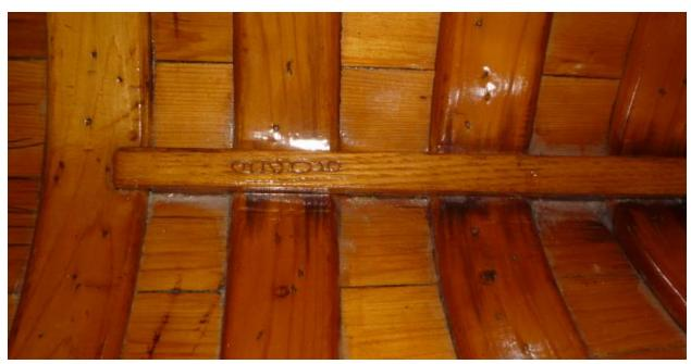
The following photos show details of the stern seat, the yoke, and the bow seat, respectively. The seats were recaned by Ralph. As is clear from the overview photo, there are no additional thwarts. The yoke is nicely carved and appears to be stamped "TEAL". I suspect this is an aftermarket modification.
