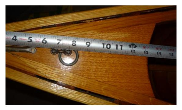
Since the rib dimensions, spacing, and chamfering seem to be important for model identification and dating, I took several photos with a ruler overlayed and did an averaging calculation. The first photo shows 9 ribs from near the center of the canoe. Rib width at the center is consistently 2 3/8 inches. The spacing between ribs varies from 1 ¼ inches to 2 inches, with most spaces being close to 1 5/8 inches. The second photo shows a closeup of a few ribs with the ruler overlayed.
