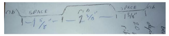
Because of the variation in rib spacing, I determined the average spacing by measuring the full length over 29 central ribs and the 29 adjacent spaces. That length was 117 inches. Given the consistent rib width of 2 3/8 inches, the average space can be calculated. It is 1.66 inches, very close to 1.625 inches, the dimension shown in the sketch above. Note that at the extreme ends the final ribs are much wider and thinner than the others.
